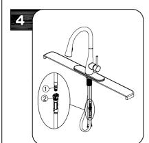
Align male fitting (1) and tabs (2) on quick connector. Push quick connector housing firmly upward and snap onto receiving male fitting. Pull down moderately to ensure connection has been made.
