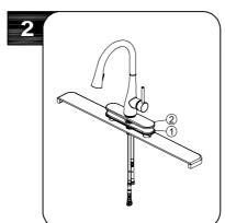
Optional Deck Plate Installation: Before installation, align the hole in the gasket (1) and deck plate (2) with the mounting hole in the sink. Place the faucet assembly through the deck plate (2) and mounting hole in the sink until the faucet assembly sets on top of deck plate (2)
