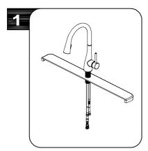
Optional Flange Installation: Before installation, place the faucet assembly through the mounting hole in sink
