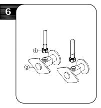
Make connections to water lines. Thread the nut (1) on the supply line onto the outlet of the water supply valve (2) and tighten with a wrench.
