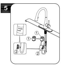
Install the weight clip (2) at the point of the hose marking "Weight here".
